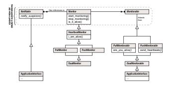
Figure 1. Class Diagram of the Object Monitoring Service Interfaces
